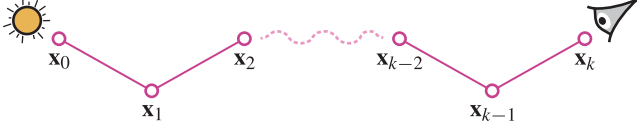
Figure 1: Regular path for length k . Vertices are fully connected from the sensor to the light sources.
