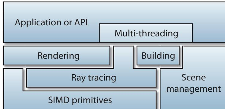
**Figure 5.1:** The multi-layer architecture of RTfact. The SIMD primitives form the basis for other generic components which are layered on top. Scene management and rendering are independent from each other and are connected through the ray tracing components. Thread management can be layered on top of the core components, or integrated into the application, which itself can be an API backend.
